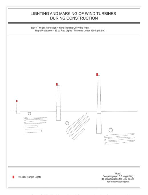
Figure A-30. Marking and Lighting of Turbines During Construction
