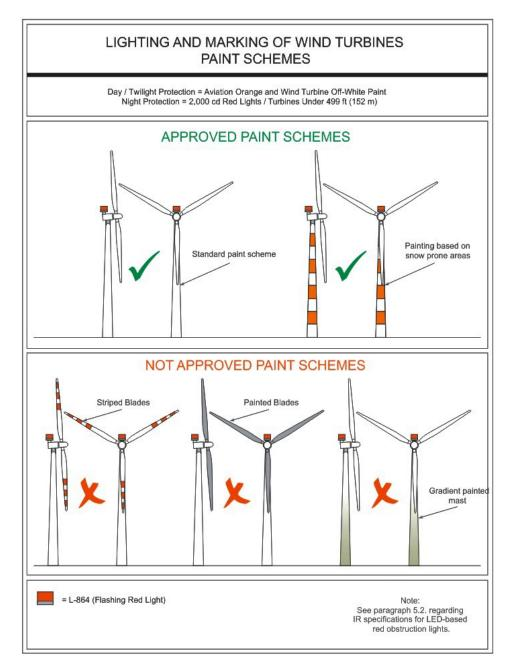
Figure A-27. Lighting and Marking of Wind Turbines – Paint Schemes
