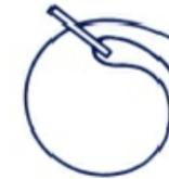
3.— REPEAT AND PASS END THROUGH A SECOND TIME, DRAW UP FREE END SNUGLY WITH PLIERS.
