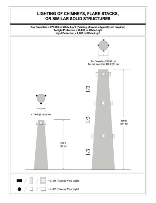
Figure A-10. Lighting of Chimneys, Flare Stacks, or Similar Solid Structures
